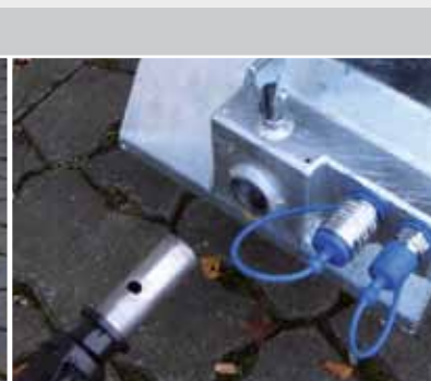
Hitch system and double-acting hydraulic connector, standard
