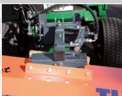
Double levelling incl. hydraulic angling
