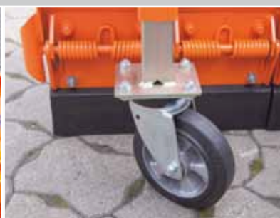
Spring flap segments (anti-icing)
