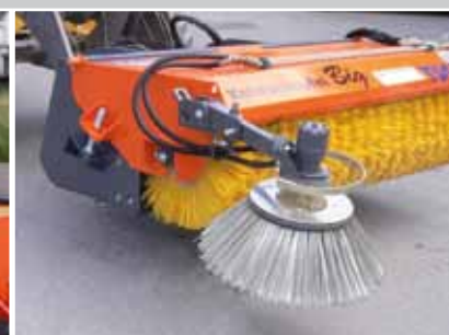
Fully adjustable hydraulic side brush (50% PP / 50% wire)
