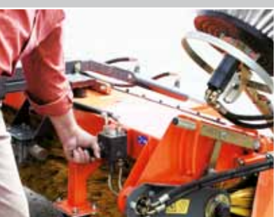
Side brush incl. speed adjustment
