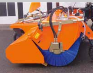
Internal motor and optimized sweeping-angle
