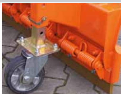
Spring flap segments (anti-icing)
