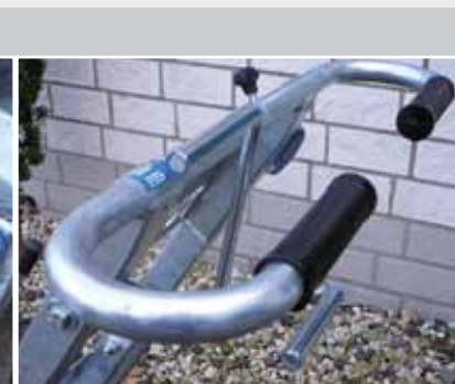
Height adjustable guiding-rod incl. forward/backwards gear
