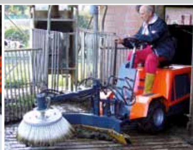
Liquid manure scraper, even in the narrowest space
