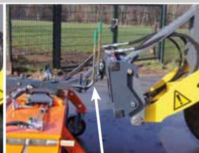
Yard loader / Front loader attachment incl. parallelogram and pendulum compensation incl. height indicator
