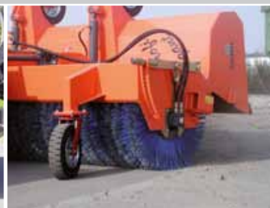
Easy brush adjustment by adjusting-lever system
