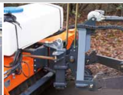
3D hitch system with roller floating tunnel
