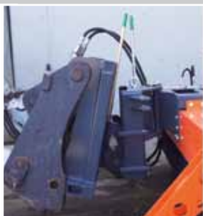
Roller floating tunnel with height indication and pendulum adapter
