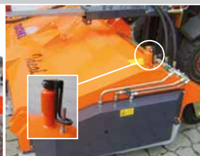
Brush adjusting lever facilitates brush adjustment
