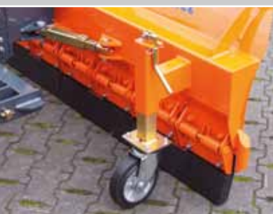
Wheels incl. infinitely variable height adjustment
