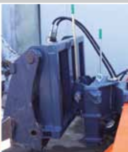
Roller floating tunnel with height indication and pendulum adapter
