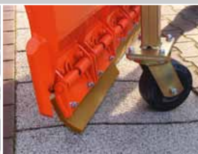
Anti-icing spring flap segments (standard)
