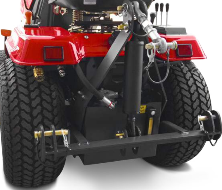
1 3-point rear attachment system
