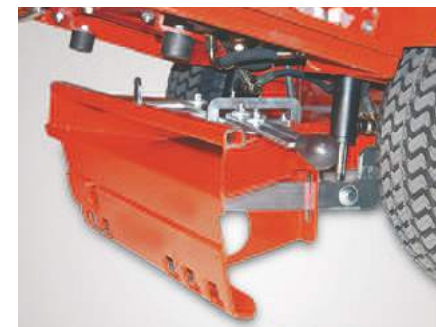
Practical coupling system for mounting all attachments without tools
