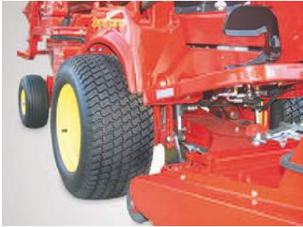
Tires especially for use on grassy surfaces ensure low pressure on the ground
