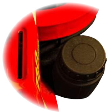
1 Filler neck for 30 liter fuel tank
