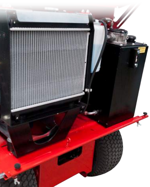
1 Water-cooled diesel engine and hydraulic tank
