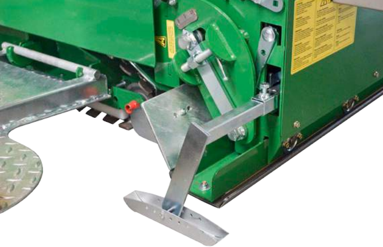
1 Integrated height levelling for evenly flat installation
