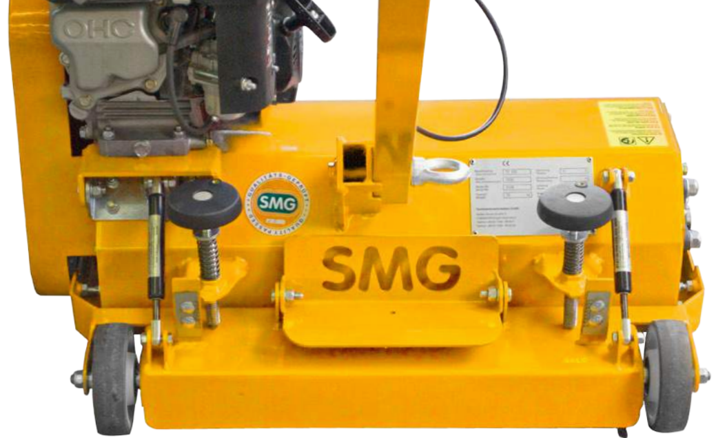
2 Working depth adjustable via spindles
