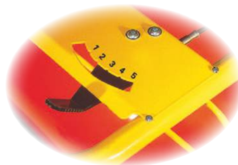
2 The quantity of granules strewn can be accurately controlled by the adjustable speed of the vibrating screen
