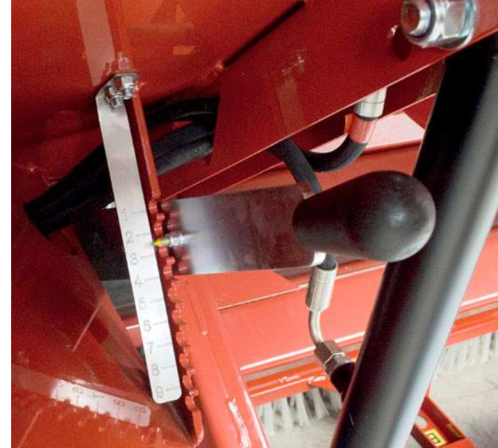
Material output can be adjusted precisely
