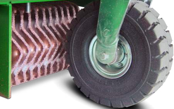
1 Milling cylinder with hard metal discs
