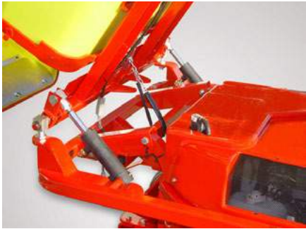
SC2D: hydraulic lifting for tipping the filter box
