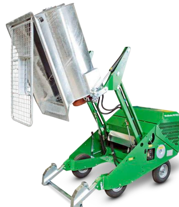
2 Container emptying in all standard dumpers
