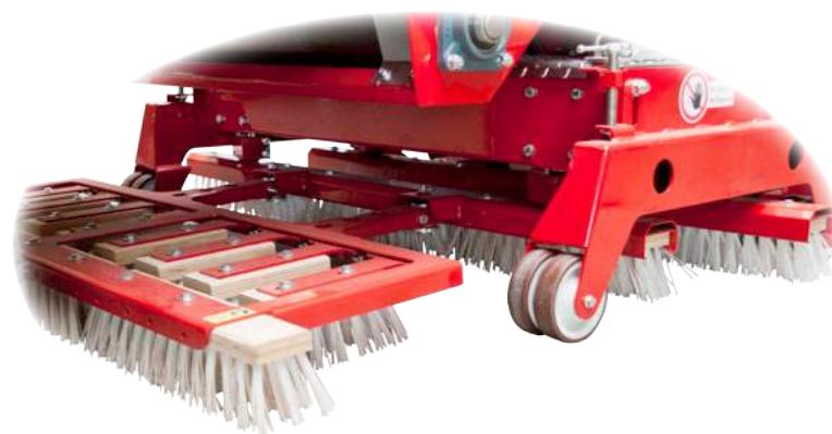
2 Brush unit for straightening and evening out the pile and brushing in the filling material
