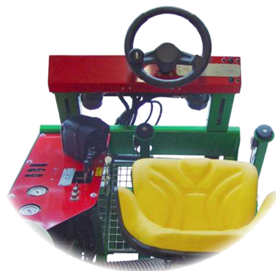
2 Operator stand with control board
