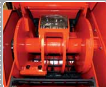
Rotor diameter 600 mm with 6 chipping blades and large flywheel.
