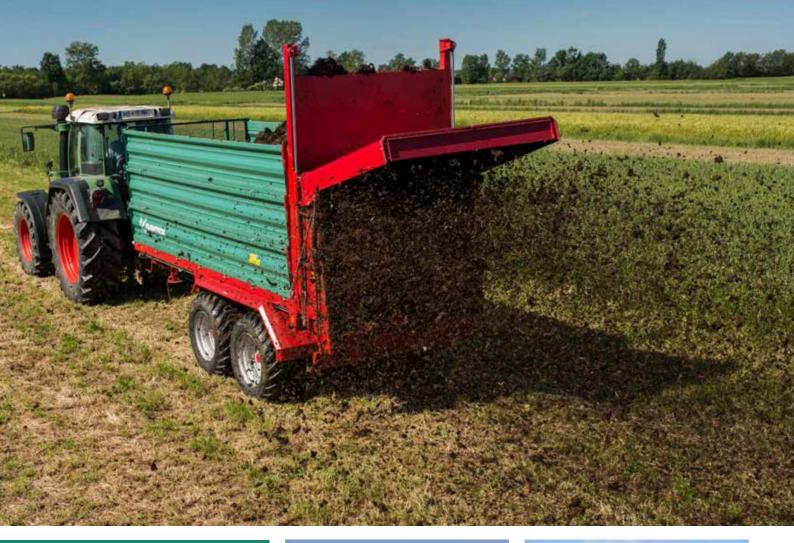
» Protective guard against dirt on the towing vehicle
