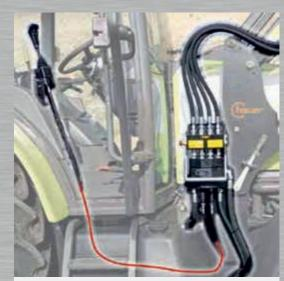
All functions with one handle. With the single-lever control unit, the loader operations can be performed even more efficiently and rationally. The monoblock valve is directly connected to the hydraulic system of the tractor.
