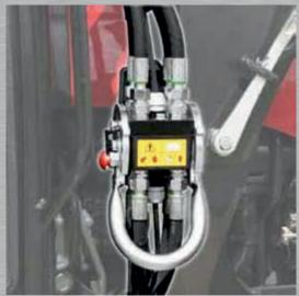
The multi-hose coupler "synchro-lock" facilitates and accelerates the joining of the hydraulic connections for the front loader. Also available with integrated electric coupling.
