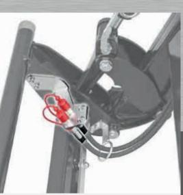
The coupling connectors for the additional hydraulic functions are mounted easily accessible on the side of the equipment quick-change device.
