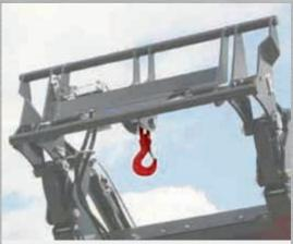
Load hook – the preparation for fastening the rotatable hook is present on the quick-change device as standard.
