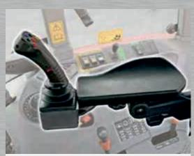
The "ELC" single-lever control unit is an electroproportional control valve for the loader functions and additional valves. As an option, a five-way adjustable arm support is additionally available.
