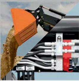
The quick dumping feature of the "VX" front loader generation additionally accelerates the emptying of the implement. The valve for this function is directly attached to the "MCV" system.
