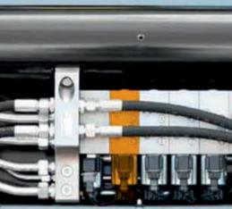
Instead of the normal coupling connector for the additional functions, a "synchro-lock" with 2 or 4 couplings is also available.
