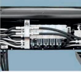
The hydraulic valve block system "MCV" is particularly characterized by central oil distribution and compact, modular design. The "MCV" can be expanded to a maximum of 4 additional hydraulic functions. The valve block is protected by a steel plate cover outside the field of vision in front of the transverse tube.
