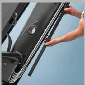
An additional advantage of the loading arm profile: the hydraulic lines are mounted under the loading arm – protected by covers. The oil supply to the "MCV" valve is by way of steel pipes.
