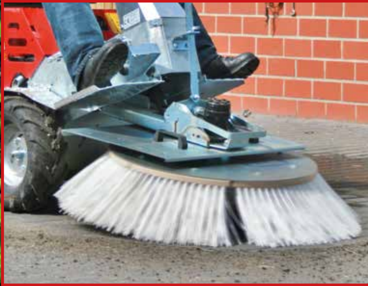
Fig.: Cleanmeleon 2 with radial brush R 1000 (PPN brush, small picture / steel brush, big picture)
