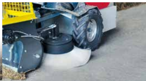
Very clean results with additional radial brush R 650.
